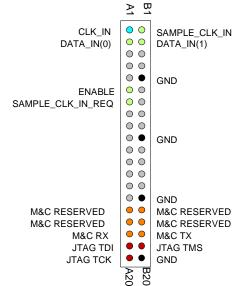
direct connection between two ComBlocks when control register REG9(4) = '0'.
