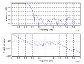
(filter response normalized for 4\*symbol rate = 40 MHz)
