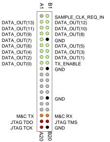
This connector is used when output data is pulled out by the next module (configuration REG9 bit 2 = 1).
