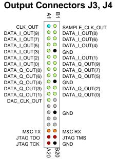
This connector is used when output data is pushed out (configuration REG9 bit2 = 0).
