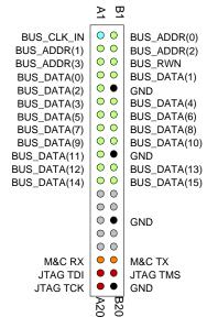
This connector is used for point-to-multipoint (bus) connection when control register REG9(4) = '1'. COM-1002 is a bus slave. It always listens to BUS\_CLK\_IN, BUS\_ADDR, BUS\_RWN.
