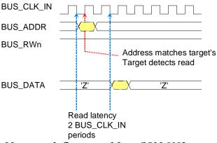
Master reads flow control from COM-1002 target
