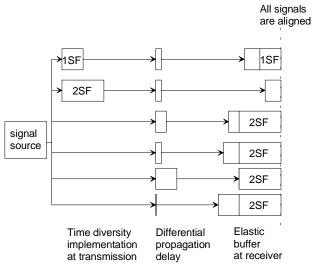
The COM-1025 software generates up to 8 differentially delayed copies. The delay is known, user-programmable and always an integer multiple of superframes.
