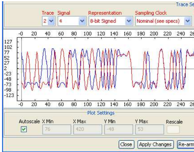
ComScope monitoring the modulator output (QPSK)
