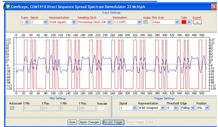
ComScope example, showing code lock with aligned: received spread signal after RRC filter (blue) vs code replica (red)
