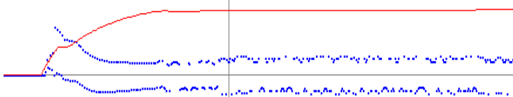
Demodulated symbols (blue trace1/signal2) AGC (red trace2/signal2) Start of frame (trigger1)
