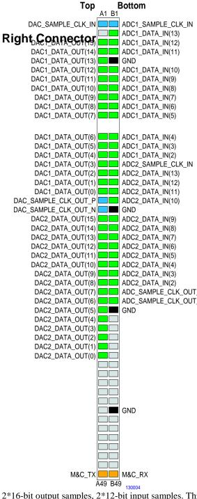
2\*16-bit output samples, 2\*12-bit input samples. This interface is compatible with the COM-3504 dual Analog<->Digital Conversions.
