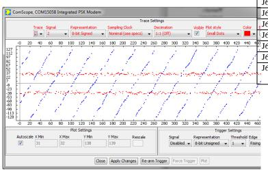
ComScope example: showing demodulated Ichannel (red) and received phase after scanning/before tracking (blue)
