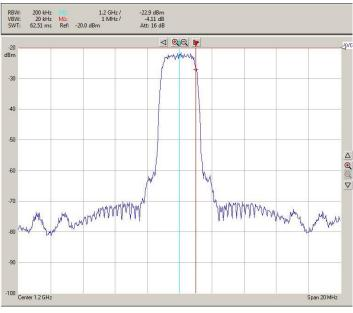
Typical RF output spectrum (after D/A conversion and direct RF modulation)
