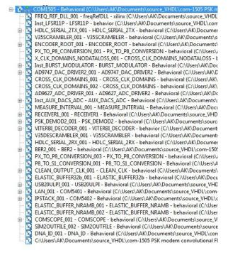
*COM1505.vhd*: top level. Includes modulator, demodulator, clock generation, interface to a supervisory microcontroller (8-bit address/data bus to exchange control registers REG and status registers SREG). CLK\_P is the main processing clock.
