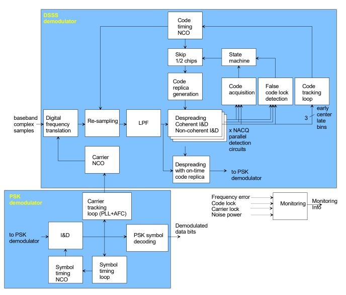
The *DSSS\_DEMOD2.vhd* component conceptually comprises two distinct and mostly independent sections: (a) a spread-spectrum receiver (code acquisition and despreading) followed by (b) a regular PSK demodulator. Architecturally, this means that the PSK modulation could be replaced with other modulation types without much effort.
