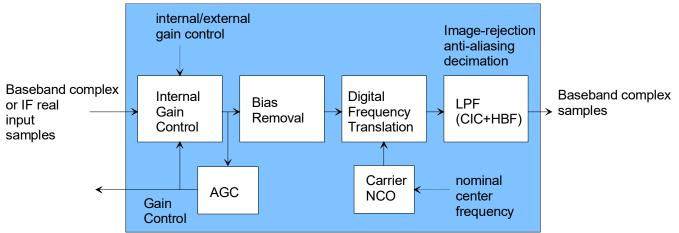
The ADC samples are first processed in the RECEIVER1.vhd component as illustrated above.
