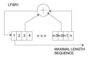
The code period is 2<sup>n</sup>-1, where n is the number of taps in the shift register. The LFRSa are initialized to all 1's at the start of each period. The LFRSs will generate all possible n-bit combinations, except the all zeros combination.
