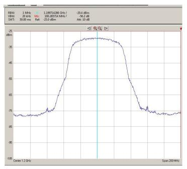
Output spectrum (after D/A conversion and RF modulation): 59.999 Mchips/s
