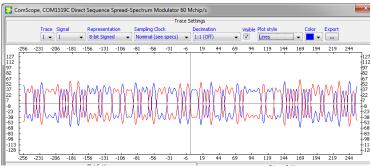
ComScope Window Sample: showing the modulated output waveform: blue for I-channel, red for Q-channel.
