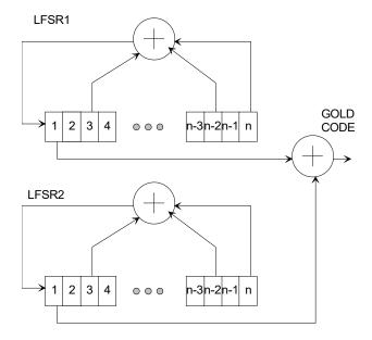
The code period is 2<sup>n</sup>-1, where n is the number of taps in the shift register. The LFRSa are initialized to all 1's at the start of each period. The LFRSs will generate all possible n-bit combinations, except the all zeros combination.
