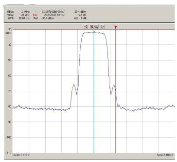
Output spectrum (after D/A conversion and RF modulation): 30 Mchips/s
