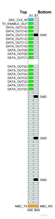
This interface is compatible with the COM-2802 DDS modulator running at 480 MHz (x8 interpolation, 60 MSamples/s at baseband, 0-200 MHz IF out)
