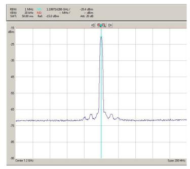
Output spectrum (after D/A conversion and RF modulation): 2 Mchips/s
