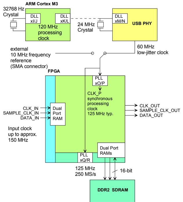
The FPGA internal frequencies are locked onto a single 24 MHz crystal oscillator. This oscillator (part of the USB PHY) serves as reference for the 60 MHz USB PHY interface clock, and the 125 MHz FPGA clocks.
