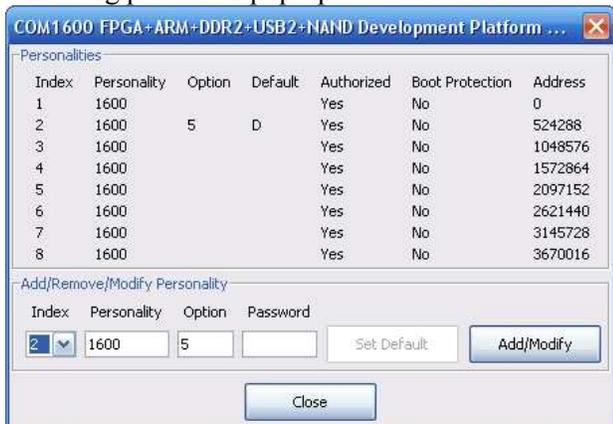
From this panel, one can select the default personality index and program the FPGA .mcs configuration file into the board flash memory.
