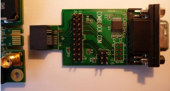
Optional adapter for programming the flash-based microprocessor via serial link to a PC, or through a 20-pin ARM JTAG pod.
