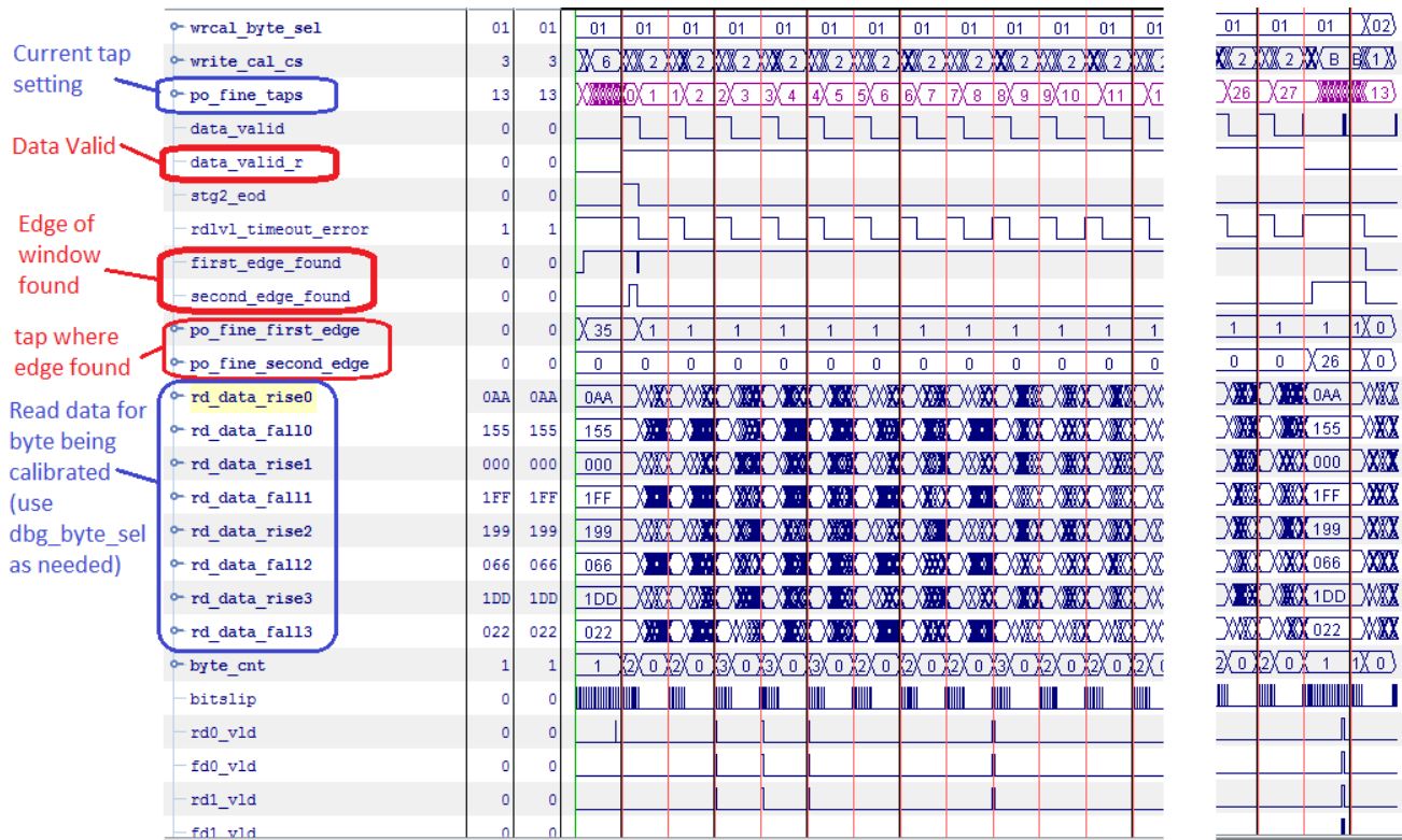
Figure 3-76: Vivado Logic Analyzer Feature Capture of Write Calibration
