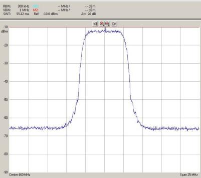
QPSK 10MSymbols/s, root raised cosine filter 20% rolloff
