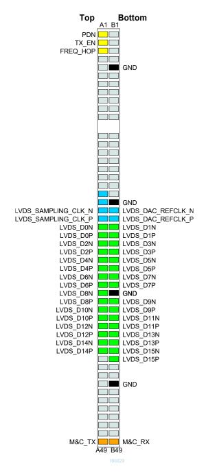
This interface is compatible with the COM-4009 RF modulator (-D firmware option)
