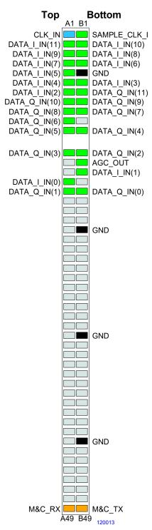
2\*12-bit baseband input samples, compatible with COM-30xx receivers (-A/-D firmware options)
