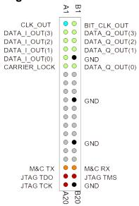
This interface emulates the COM-1001 demodulator output. (-G firmware option)
