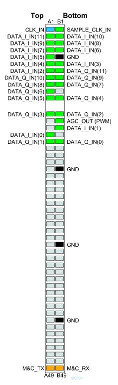
2\*12-bit baseband input samples, compatible with COM-30xx receivers (-B firmware option)
