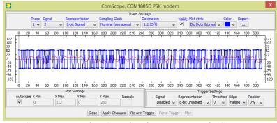
ComScope Window Sample: showing internal PSK *demodulator signals (blue = center of symbol,* red = baseband received waveform)
