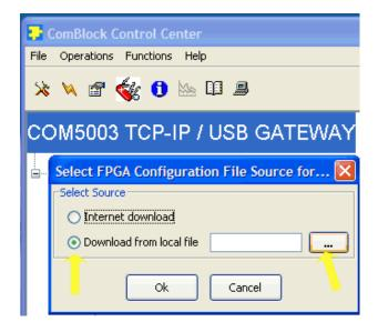
The software configuration files are named with the .bit extension. The bit file can be downloaded via the Internet, from the ComBlock CD or any other local file.
