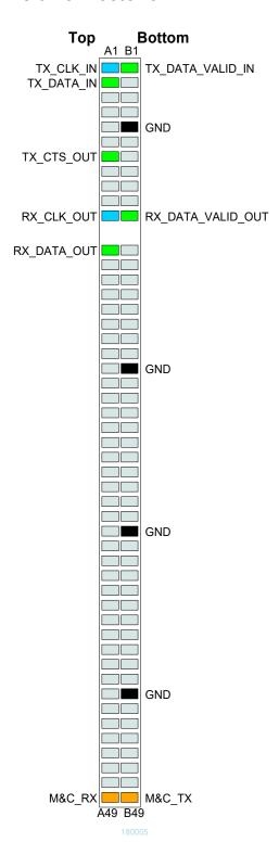
Modem synchronous serial input/output data, compatible with other digital ComBlock modules (COM-1800, etc). (-B/-C firmware options)
