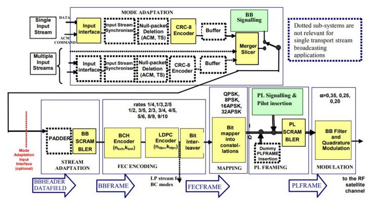
Figure 1: Functional block diagram of the DVB-S2 System
