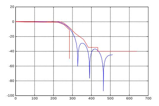
The Matlab program <code>/matlab/dvbs2\_firrcos.m</code> is used to generate the FIR coefficients and verify compliance with the spectral mask
