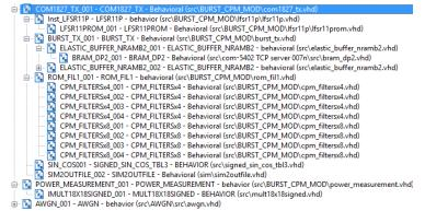
*COM1827\_TX.vhd* generates complex baseband continuous phase-modulated samples from byte-size input data.
