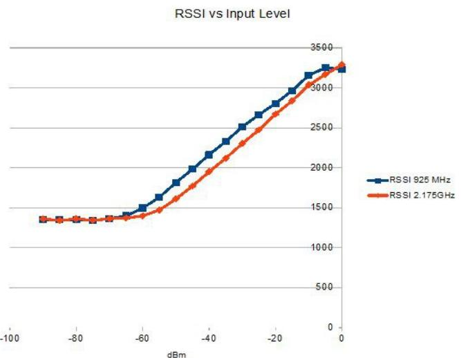
Note: RSSI measurement below -50Bm is affected by the presence of 10 MHz frequency reference when supplied to an external LNB (see control register REG46(2)).
