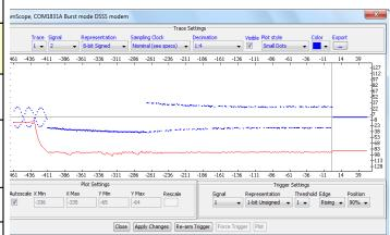
wing trace1 signal2 (in blue): ng preamble (left) then data (right in red) shows the I-symbol tracking
