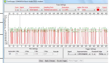
ComScope example, showing code lock with aligned: received spread signal after RRC filter (green) vs code replica (red)
