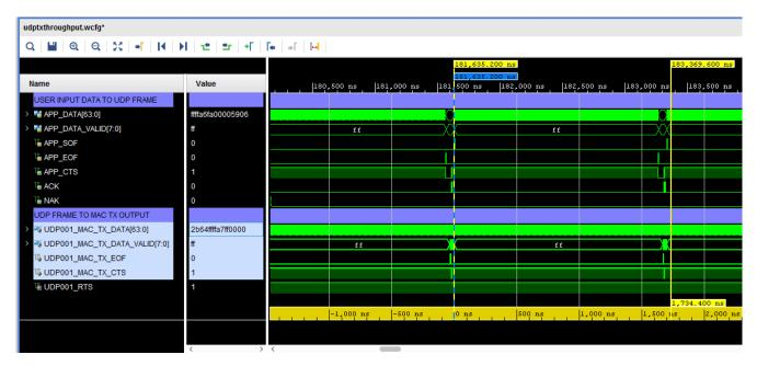
For example: in the case of a 2048-byte frame, the transmit latency is 1.734us
