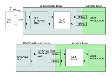
At 10G speed, the COM-5503SOFT uses the same 156.25 MHz clock as the 10G Ethernet MAC. If the user application uses a different clock, dual-port RAMs must be used to cross the clock domain
