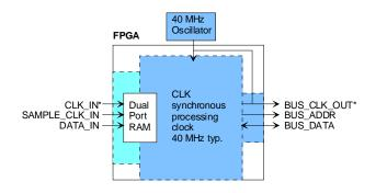
Baseline clock architecture Light blue = user defined input clock Darker blue = internal 40 MHz clock \* indicates edge-trigger signal
