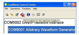
The personalities window opens and displays all configurations, options and authorization. The default configuration (identified with a 'D' in the Default column) is the one loaded at power up or reset into the FPGA.
