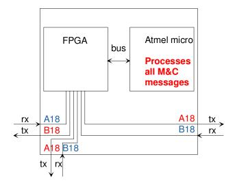
In ComBlock FPGA development platforms, messages also go through the FPGA. It is thus mandatory to follow two rules when writing custom code for the FPGA:
