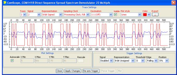
3. Demodulated signal shows near perfect constant amplitude. . [COM-1418 comscope: trace 1 signal 3]
