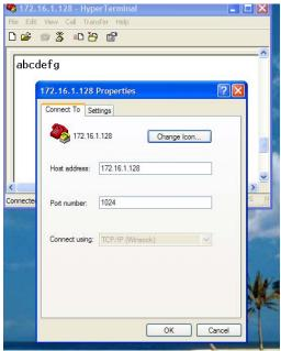
Configure the sending Hyperterminal with "TCP-IP (Winsock)" connection, IP address as the first COM-5003 IP address, port number 1024. Then configure the settings as shown below:
