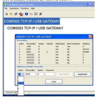
Do not reboot now, as the other COM-5003 must also be switched from USB to TCP-IP gateway. Once both COM-5003 are configured as TCP-IP gateways with new IP addresses, recycle power on the ComBlock assembly to enact the IP address changes.
