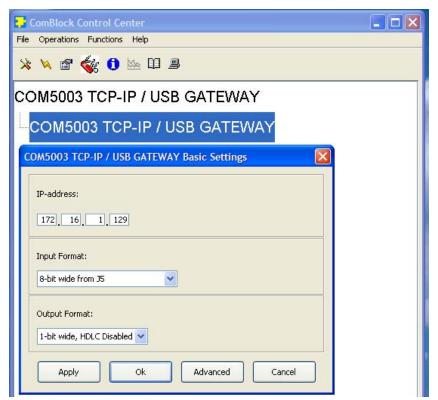
Configuring the second COM-5003 in the transmission link. Press OK when done. The IP addresses are configured.
