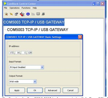
Configuring the first COM-5003 in the transmission link. Press OK when done.
